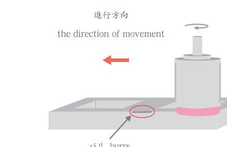
If there are too much shear drop, lower the brush vertically without rotation. Adjust the cutting amount by reducing the number of rotations, and set the grinding feed rate at a high speed.
